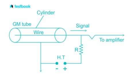
This device used to detect and measure the rate of emission of  $\alpha,\beta$  particles it consists of a cylindrical metal tube (cathode) and central wire which is anode the anode is filled with Argon gas can reduce pressure (0.1atmp) an potential difference of nearly1000v is apply across the electrodes when  $\alpha$  or  $\beta$  particles enters the tube through the mica window it ionizes the Argon atoms.
