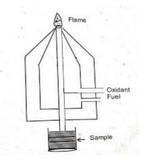
Sample solution, fuel gas and oxidising gas are passed through separate inlet and mixed at the top of the flame. Sample solution is converted to tiny droplets, which on evaporation form residue and residue finally produce ground state atoms.
