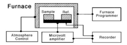
Block Diagram of the DTA apparatus consists of the following components
