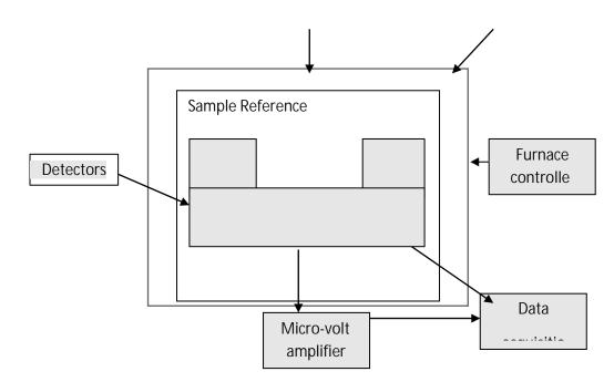
Detector: In case of detector thermocouple is used to measure the temperature change while the sample heated under controlled environment. For the case of low temperature copper- constantan or cromel alumel thermocouple is used and for the case of corrosive atmosphere or high temperature pt/13%rh thermocouple is used.
