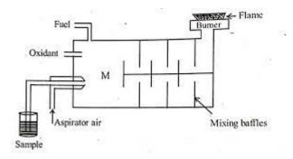
Sample solution, fuel gas and oxidising gas are mixed in mixing chamber This mixture is then passed through a series of baffles where thorough mixing and formation of uniform droplets of the sample take place.
