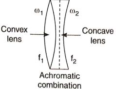
Consider two lenses of focal lengths  $f_1$ ,  $f_2$  and dispersive powers  $\omega_1$ ,  $\omega_2$ . If f is the combined focal length of the system, then
