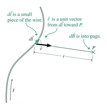
Let 'dl' the length of one such element and 'r' be the displacement vector from the point 'P' to the element. Biot – Savart observed that the magnetic induction 'dB' at point 'P' due to small element of the current carrying conductor depends upon the following factors
