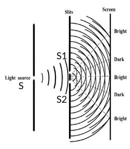
When the crest of one wave falls on the crestof another or trough of one wave falls on the trough of another, they mutually reinforce each other and the amplitude increases. Hence intensity which is proportional to square of the amplitude is maximum. So maximum brightness is produced. This is known as **Constructive Interference**.
