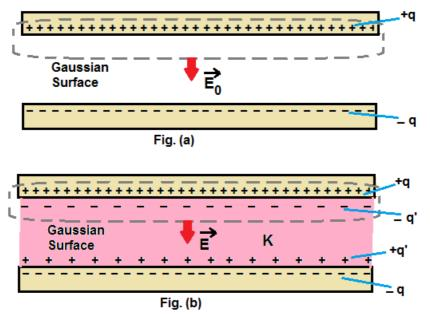
Here, the charge on either plates is 'q'. The electric field direction is as shown in the figure i.e., from positive plate to the negative plate. From Fig.(a), using Gauss law and its applicability, one can write,
